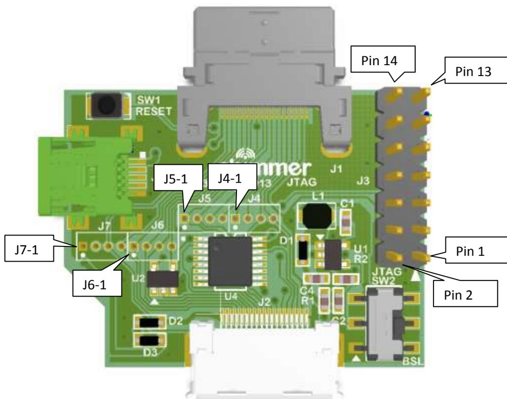
Figure 2-4: Shimmer3 JTAG Developer Board Top View
