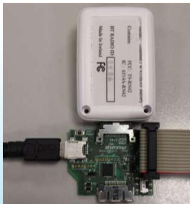
Figure 2-2: The Shimmer3 JTAG Developer Board should be powered by either the (a) Shimmer Dock or (b) the on-board Mini-USB connector.
