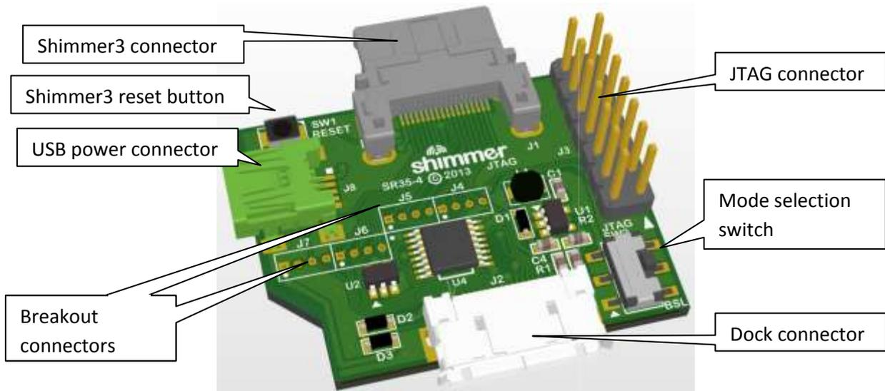
Figure 2-1: The main features of the Shimmer3 JTAG Developer Board.
