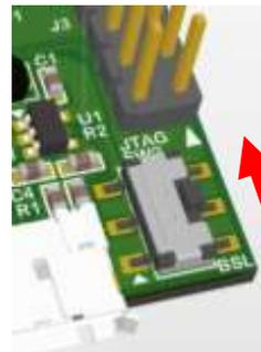
Figure 2-3: Mode selection switch actions - (a) Normal Dock Mode for and (b) JTAG Programming Mode
