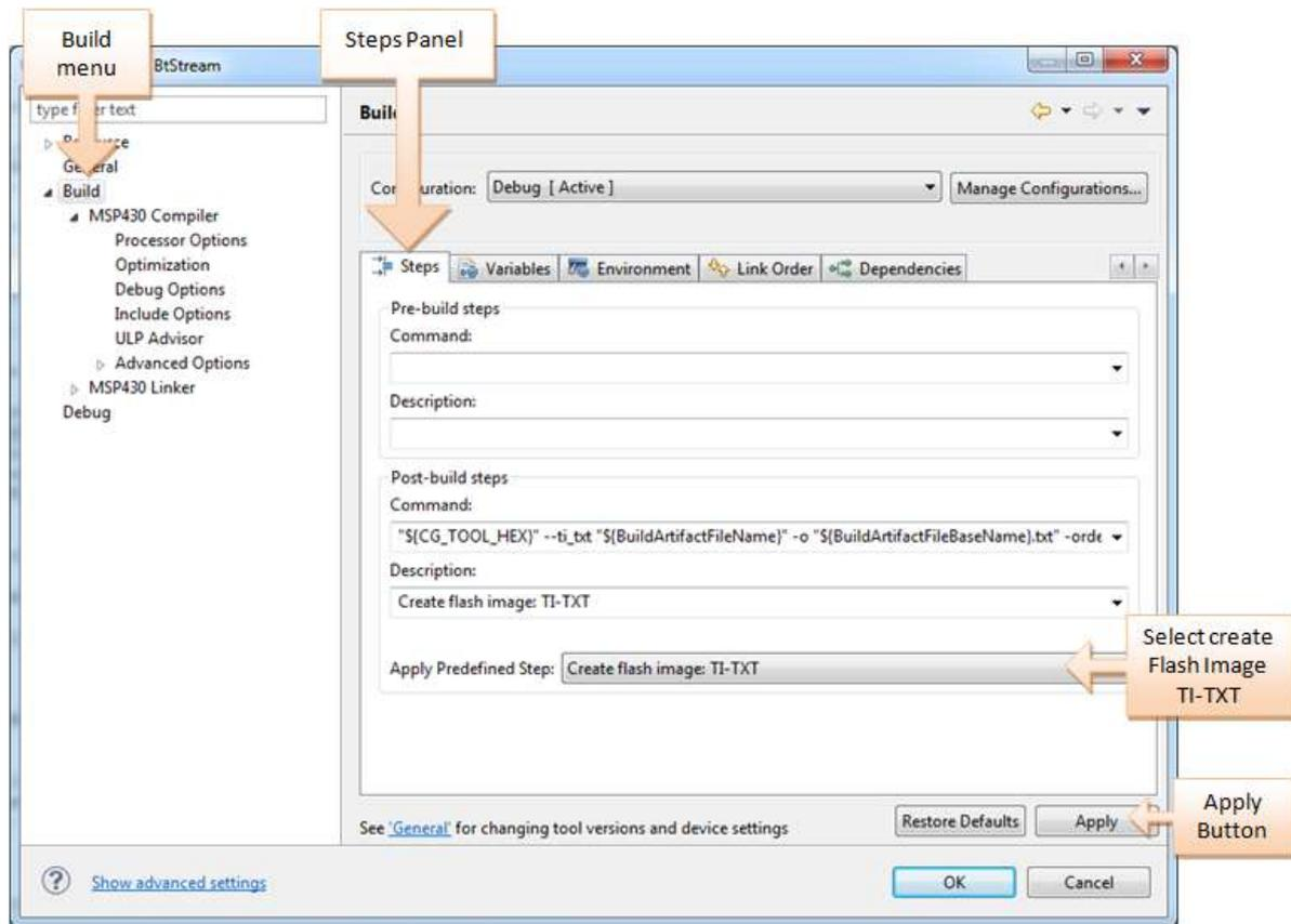
Figure 4-1: Creating an output TXT file using Code Composer for custom firmware programming with Consensys.
