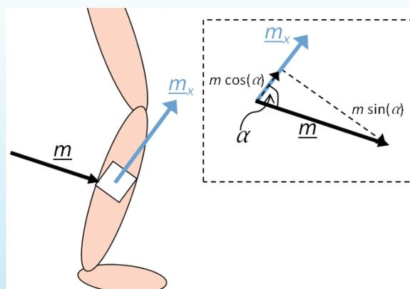
Figure 3-8: Uni-axial magnetometer attached to a leg segment
