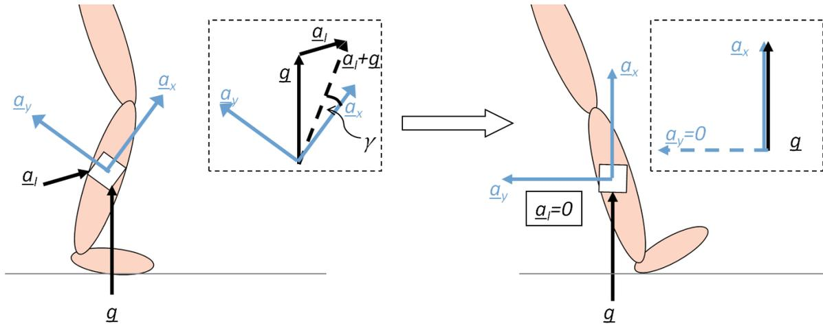
Figure 3-6: Bi-axial accelerometer attached to a leg segment
