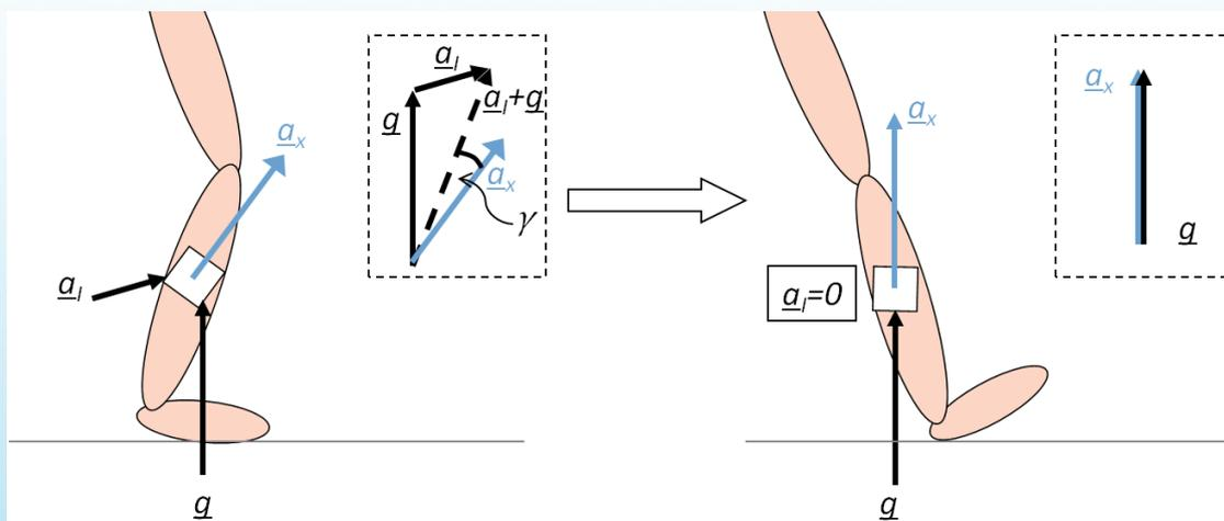
Figure 3-5: Uni-axial accelerometer attached to a leg segment
