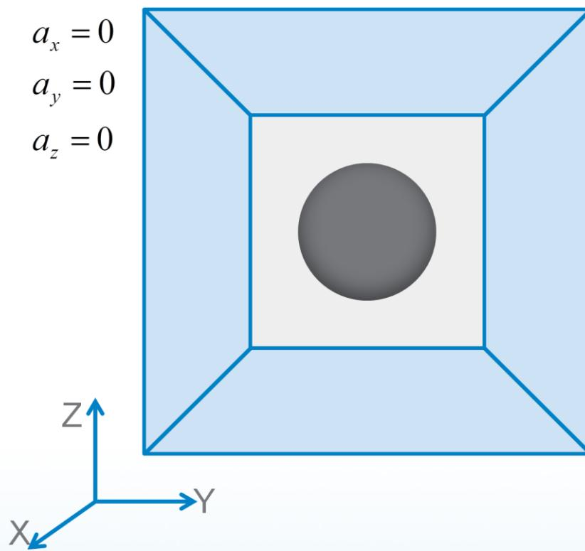
Figure 3-1 Accelerometer in free-fall
