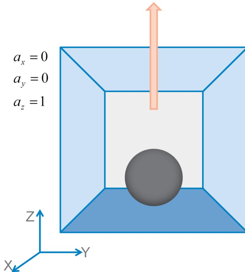
Figure 3-3 Accelerometer measuring gravity in upward positive Z-direction
