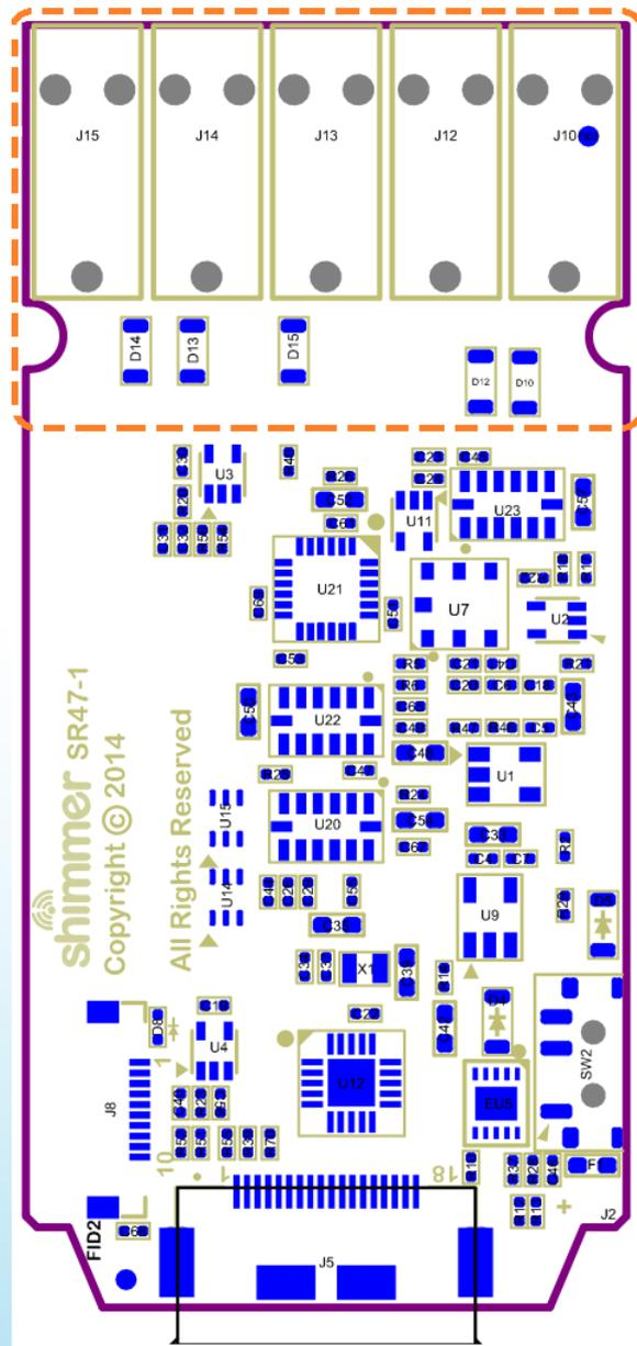
Figure 6-1: EMG Board Layout (bottom view)
