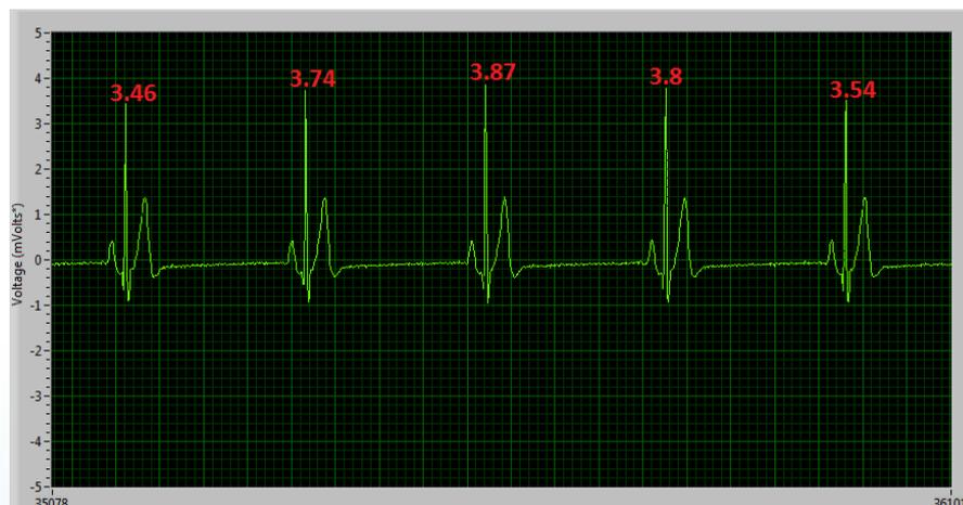
Figure 4-3: 30 BPM ECG signal sampled at 102.4Hz, showing high R wave height variation.
