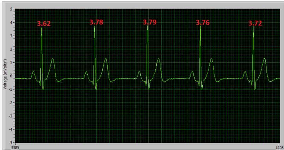
Figure 4-4: 60 BPM ECG signal sampled at 204.8Hz, showing reduced R wave height variation.
