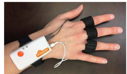
Figure 2. Shimmer3 GSR sensor setup on participant's non-dominant hand.
