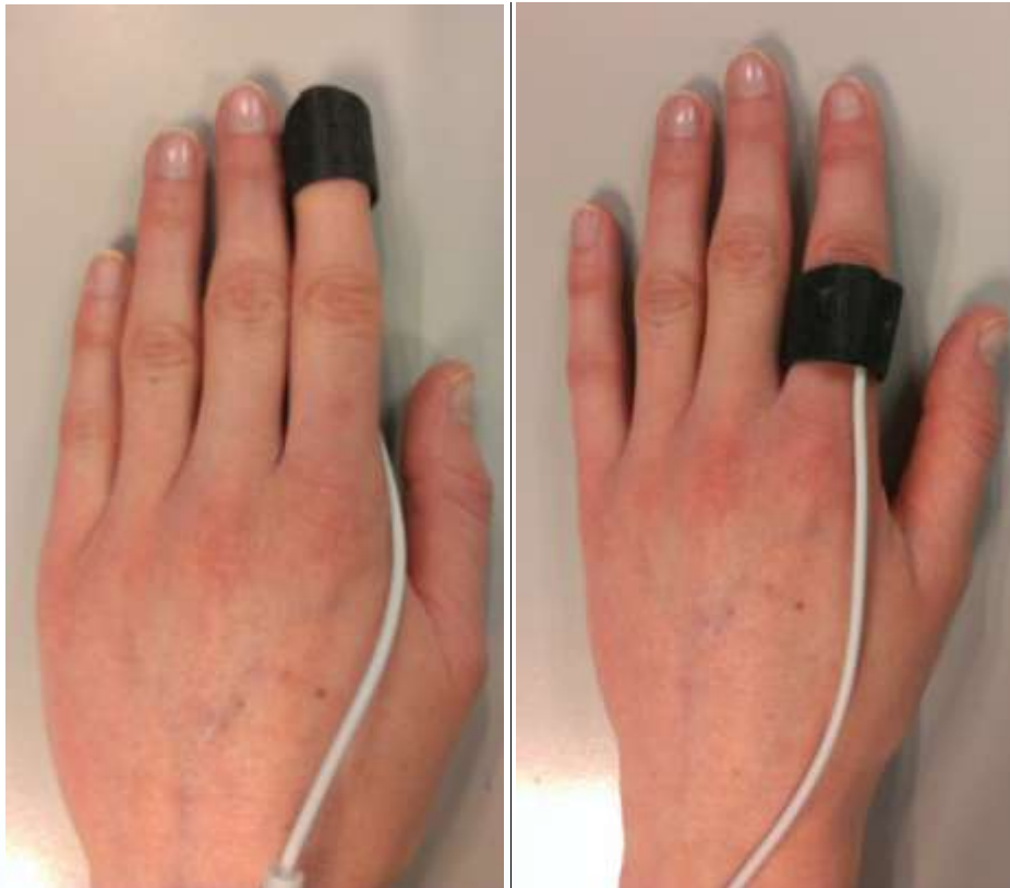
Figure 3-2: Example finger sensor positioning for Optical Pulse measurement
