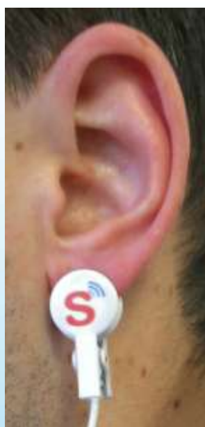
Figure 3-1: Ear-lobe sensor positioning for Optical Pulse measurement
