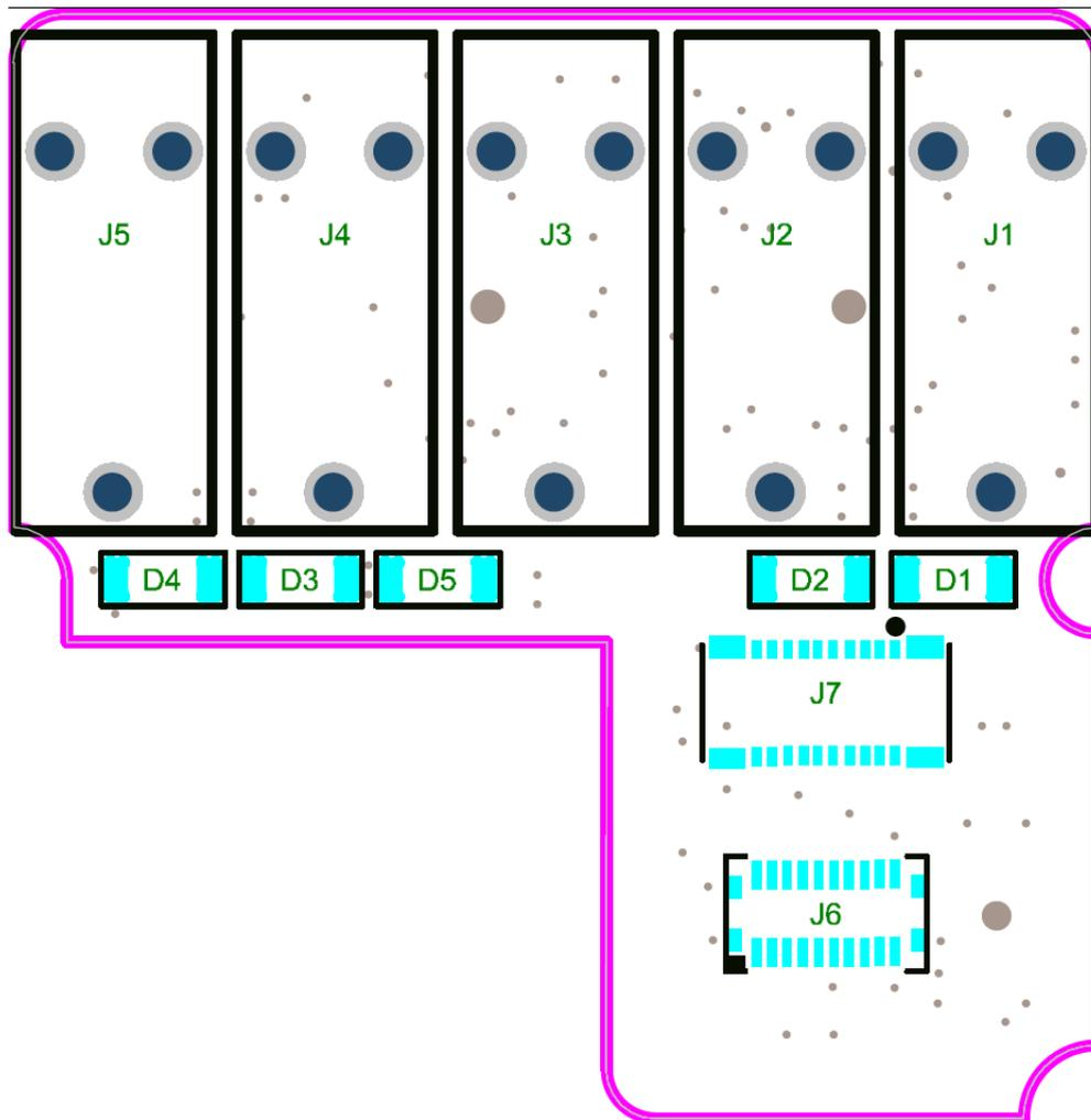
Figure 10-2 EMG Board Layout (top view)
