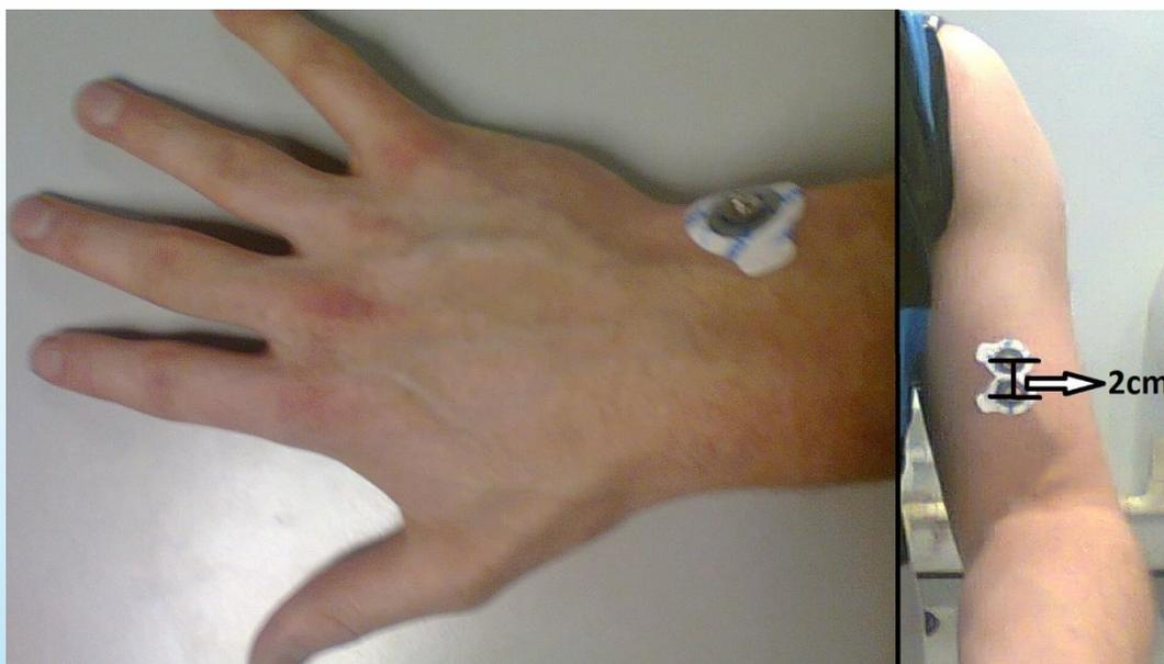
*Figure 3-2: Example positioning of the electrodes for EMG measurement.*
