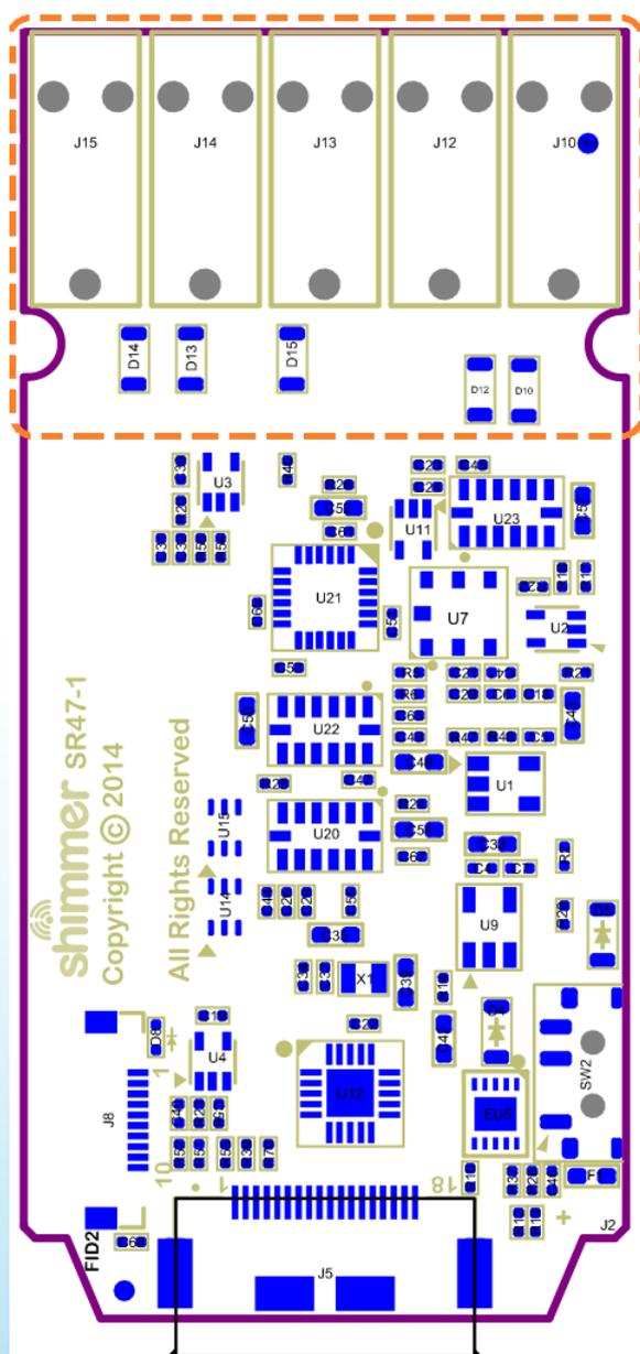
Figure 6-1: EMG Board Layout (bottom view)
