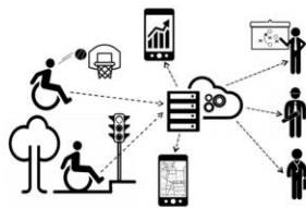
Schematic overview of wheelchair tracking, data transfer, cloud analysis, individual output display and possible future database use by athletes and coaches.
